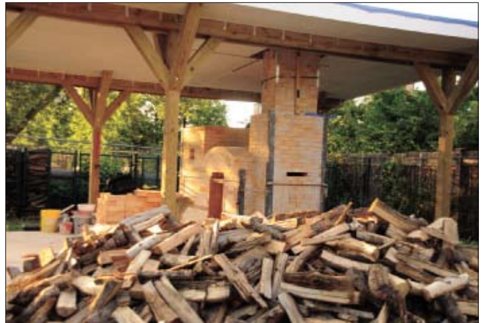
MCC_Kiln_wood.jpg – Middlesex Community College's smokeless, wood-fired Cambodian ceramics kiln was built on the grounds of Lowell National Historical Park for college and community use.
